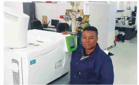
WearCheck transformer laboratory technician, Zamaswazi Dlamini, operates the new high-speed gas chromatograph (GC) at the company's Durban laboratory.
