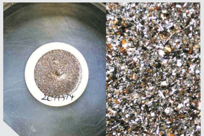
Aluminium and clutch pack material from a transmission
