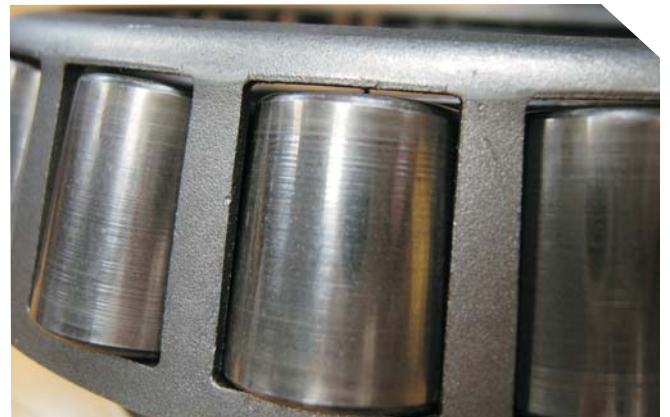
Score marks evident on the left hand outer wheel bearing rollers of a MAN F2000 26442 truck.
