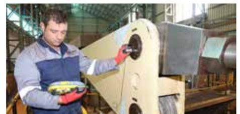
AFS technician Jaco Venter, of WearCheck, conducts ultrasonic testing of fulcrum plate pins
