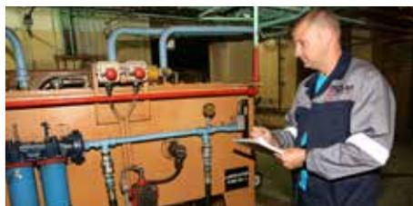
Here, Joe Kies measures the working stroke of the brake cylinder
