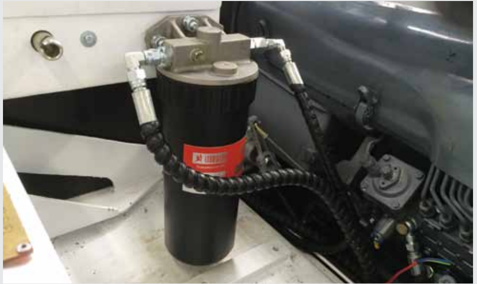
Bolted externally onto the machine is one of WearCheck's bypass filters for the transmission. The filters have already saved a mine over R1.5 million during an initial trial process
