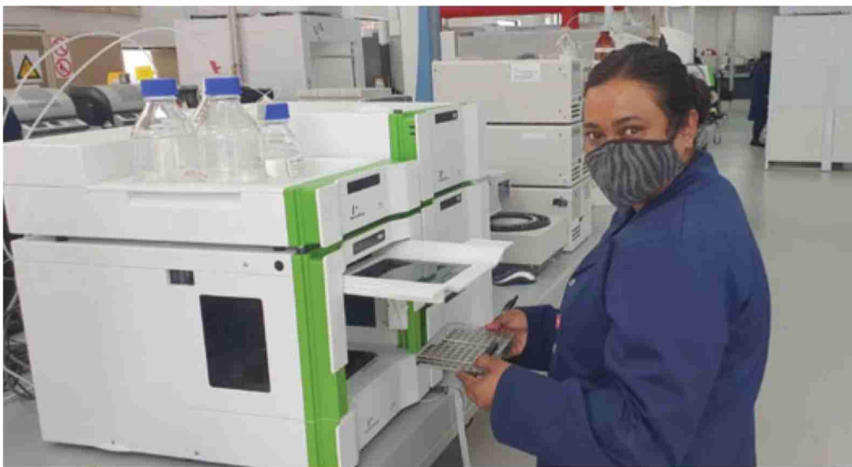
Senior analytical chemist, Lynette Pillay, feeds samples into the new HPLC (high performance liquid chromatography) machine at WearCheck's transformer laboratory in Durban. SOURCE | WEARCHECK
