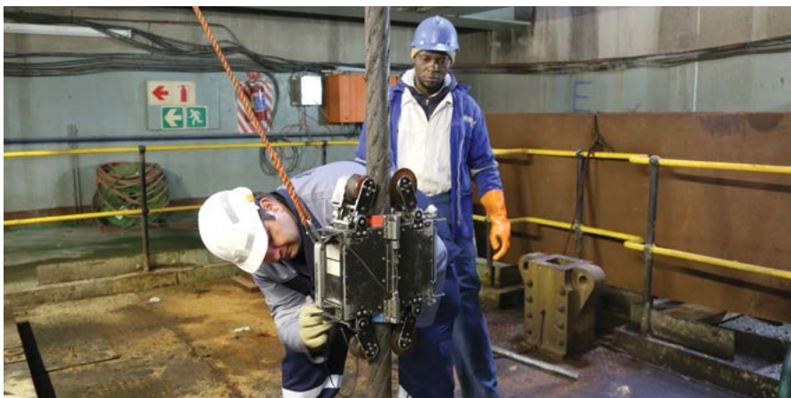
Roger Herrwood performing a rope condition assessment (RCA). WearCheck now has a technical inspection and compliance division accredited to certify the safety of hoist systems, fans, electrical panels and other critical mining systems.
