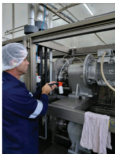
Here, an oil sample is taken from a motor-driven centrifugal pump by WearCheck onsite sampling technician, Jaco de Beer
