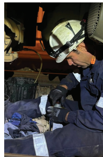
WearCheck onsite sampling technician, Jaco de Beer, takes an oil sample from a transformer
