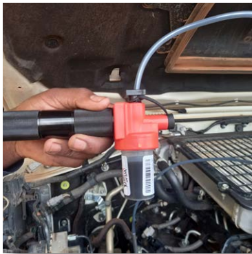
Seen here is the WearCheck oil sample pump - an instrument used for sampling at the Teichmann Group's client site in the DRC
