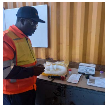
A Teichmann Group technician prepares the oil sample for submission to WearCheck for analysis
