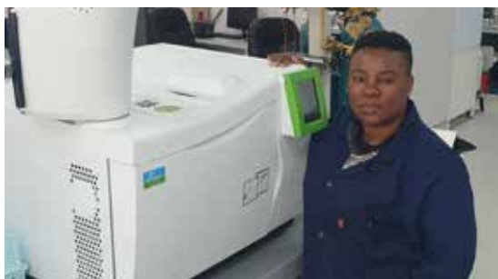
WearCheck transformer laboratory technician, Zamaswazi Dlamini, operates the new high-speed gas chromatograph (GC) in Durban. The GC, one of two new ones, has more than doubled WearCheck's capacity for processing dissolved gas analysis DGA on transformer oil samples
