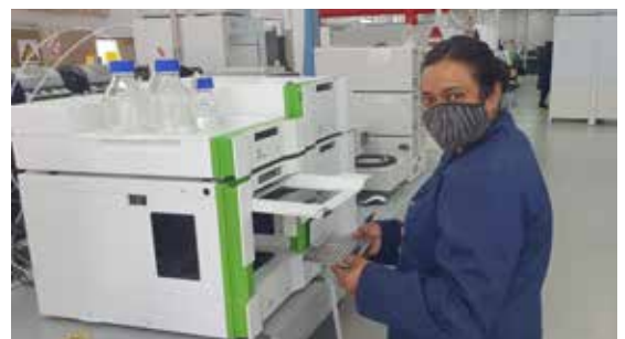
Senior analytical chemist, Lynette Pillay, feeds samples into the new HPLC (high performance liquid chromatography) machine at WearCheck's transformer laboratory in Durban
