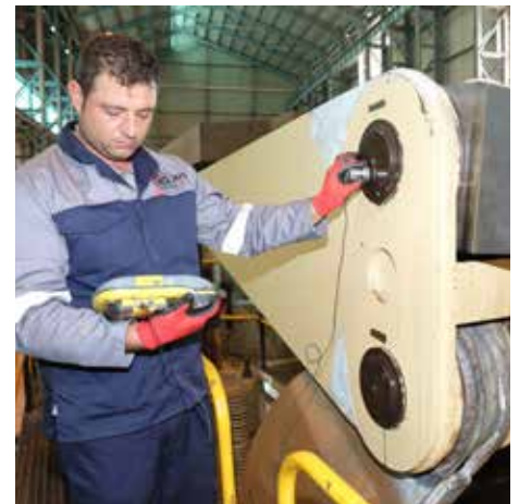
WearCheck's senior machinery inspector, Jaco Venter, conducts ultrasonic testing on a winder's brake components during a non-destructive testing (NDT) routine
