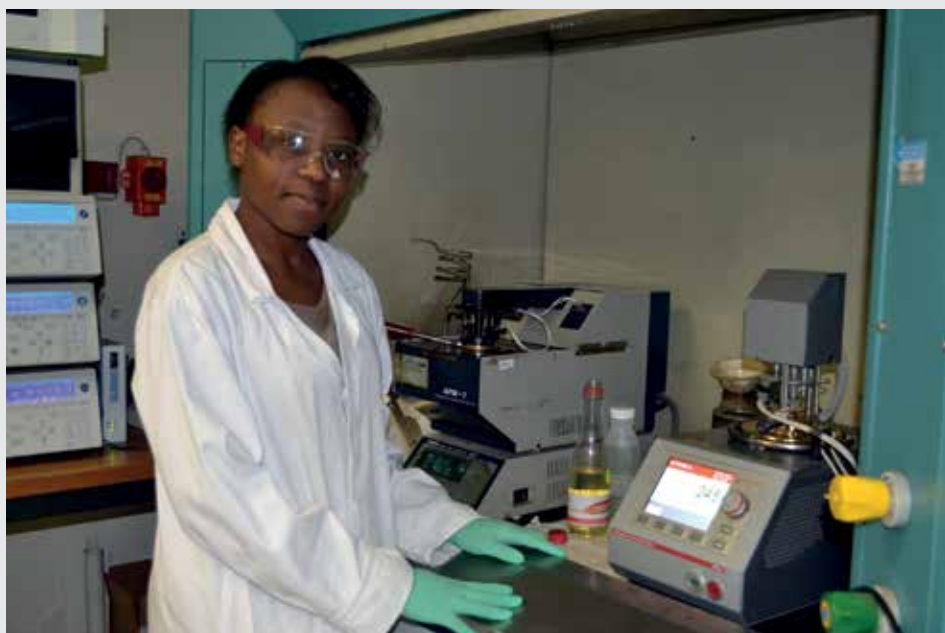
Here, senior laboratory technician Lizzy Chabangu operates the brand new PMA5 Pensky Martens closed cup flashpoint tester
