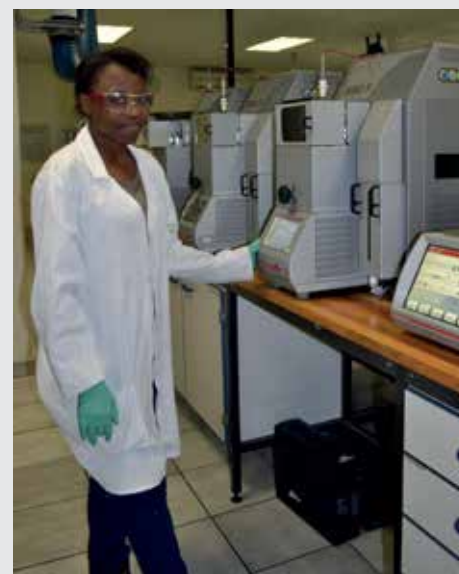
WearCheck continues to lead the way in the condition monitoring arena and boost productivity, this time by investing in the latest international laboratory technology in the form of several new instruments. This new ADU5 distillation unit is operated by senior lab technician Lizzy Chabangu
