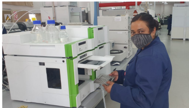
Senior analytical chemist, Lynette Pillay, feeds samples into the new HPLC (high performance liquid chromatography) machine at WearCheck's transformer laboratory in Durban.
