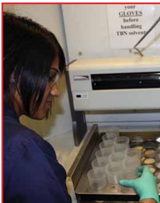
A Total Base Number (TBN) machine in operation in a WearCheck laboratory
